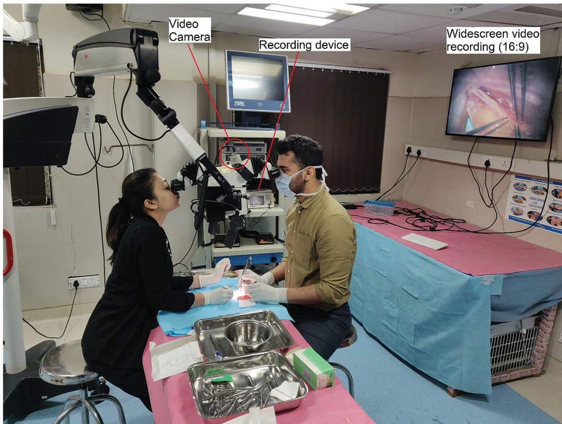
Figure 1. Training setup. Operating microscope with recording camera attached on one port, recording device, and screen in the background.
