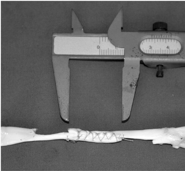
**Figure 1.** A porcine FDP tendon lengthened with a 3 cm overlap prior to loading testing. The single sutures at the ends were used to measure the lengthening of the construct at 100 N.
