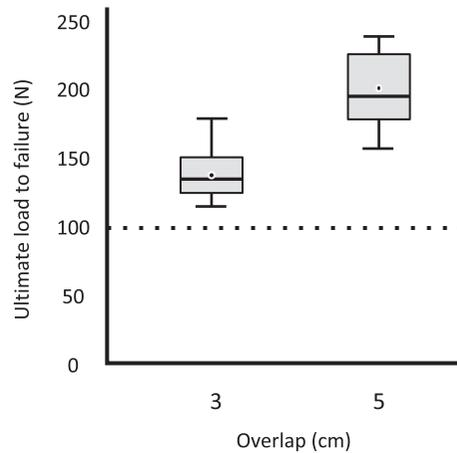
**Figure 4.** Ultimate load to failure. Twenty tendons were operated with an overlap of 3 cm, and another twenty with an overlap of 5 cm. Bars represent medians, dots means, boxes the interquartile range and whiskers the minimum and maximum loads. The dotted line represents the highest maximum force generated by forearm muscles.
