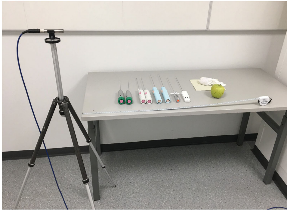
Figure 1. Set-up for laboratory measurements. The biopsy device and target were hand-held during the biopsies. The distance from the microphone was measured with the ruler on the table.
