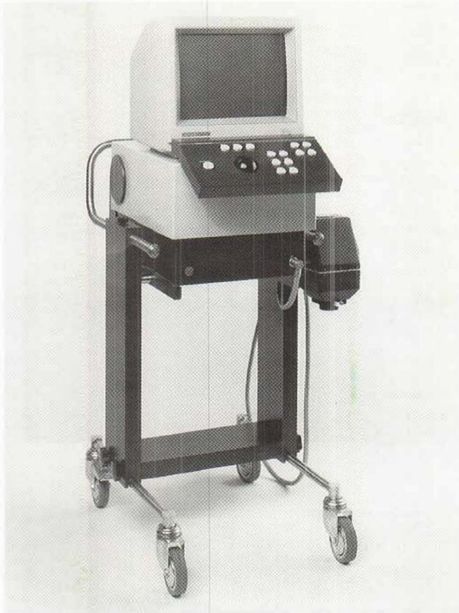
Fig. 13. 20 MHz ultrasound A,B,C,M-mode scanner (DermalScan C®, Cortex Technology, Hadsund, Denmark) for cross-sectional imaging of skin and computerized image analysis. Images are shown in Fig. 14.
