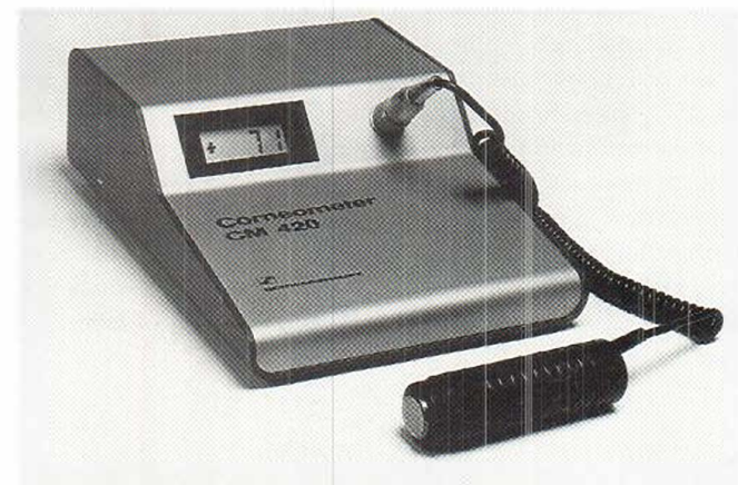
Fig. 6. Skin hydration measurer (capacitance) developed to measure dryness of skin (Schwarzaupt, Cologne, Germany, more recently Courage and Khazaka GmbH, Cologne, Germany). The apparatus measures hydration more deeply in the epidermis.
