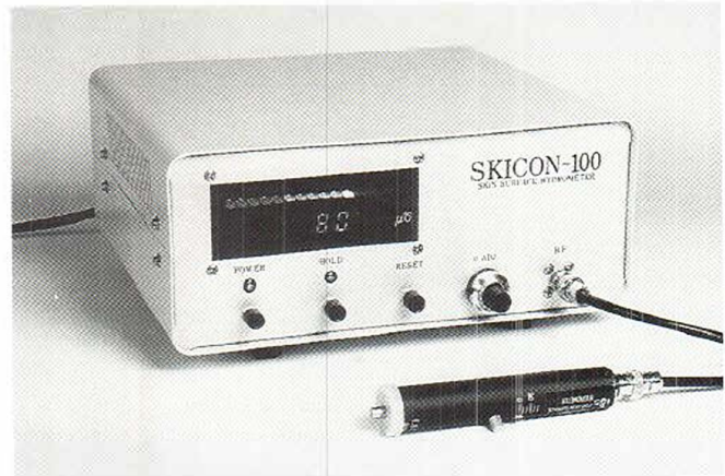
Fig. 5. Skin hydration measurer (conductance) described by Tagami and co-workers as a prototype for measurement of water absorption-desorption, Skicon-100® (IBS Ltd, Tokyo, Japan). The apparatus measures hydration superficially in the epidermis.
