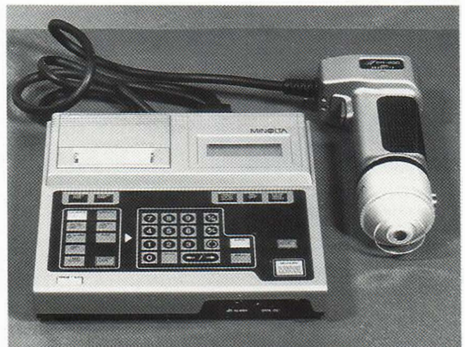
Fig. 3. Minolta Croma Meter CR-200® (Minolta, Osaka, Japan) for tristimulus analysis of colour according to the CIE system. The apparatus may be set to express colour in other coordinate systems.
