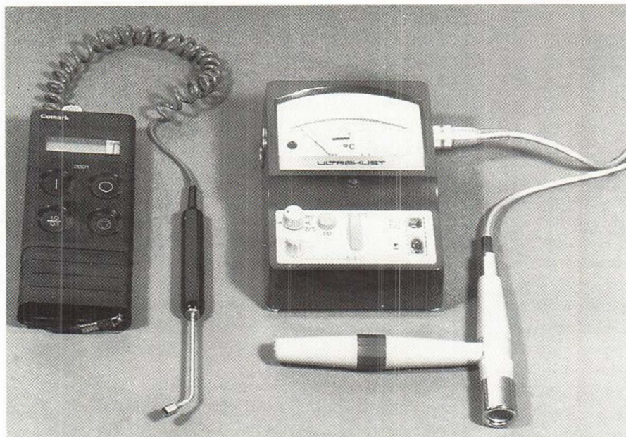
Fig. 9. Contact thermometer (Comark 2001®, Rustington, England, left) and infrared thermometer (Thermophil 203®, Ultrakust GmbH, Ruhmannsfelden, Germany) for measurement of skin surface temperature.
