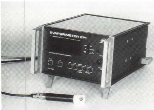
Fig. 8. Evaporimeter EPI® (ServoMed, Kinna, Sweden) for measurement of transepidermal water loss.
