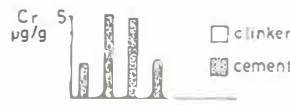
Fig. 3. Water-soluble chromate in clinker before and after adding of gypsum (cement = clinker + gypsum).
