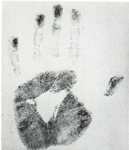
Fig. 1. Corrosion test on sheet of mild, unpolished steel. Left: print made by a 'ruster'; right: print made by one of
