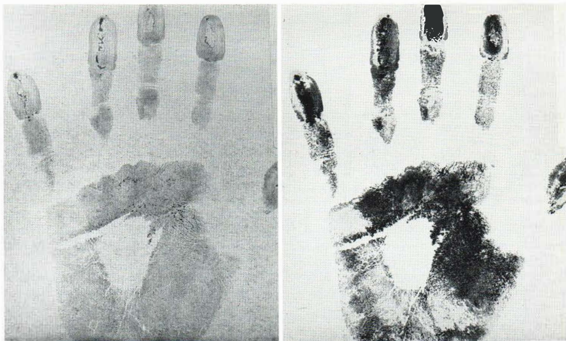
Fig. 2. Corrosion test (stage 2) on a 'ruster' carried out on sheet of 'mild', polished steel. Photograph taken 2 weeks (left) and 2 months (right) after the print was made. Corro-
