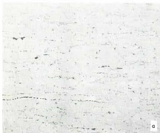
Fig. 1. Metallographic structure. (a). Type 1 steel ( \times 210 ). The very low carbon content makes the structure ferritic (pure iron). (b). Type 2 steel ( \times 210 ). The carbon content of 0.41% gives a structure with pearlite (iron and
