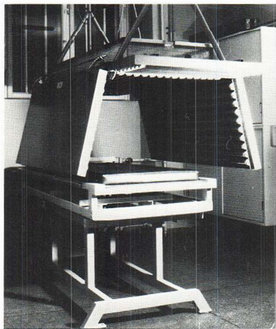
Fig. 2. UVA light source consisting of thirty-six 40 W and twelve 20 W black light tube lamps (Philips TL/08).
