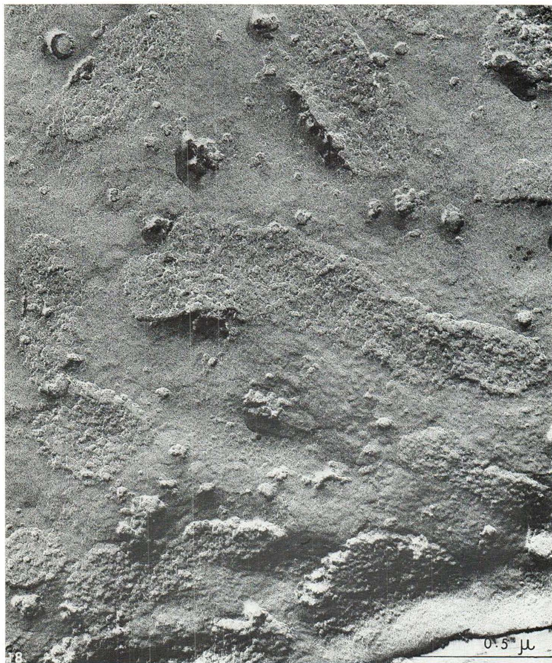
Fig. 18. High magnification of a replica of a surface horny cell shows round, oval or elongated macules. Individual macules consist of cobblestone-like particles. These macules measure on average 0.4\text{--}0.8\text{ }\mu\text{m} in long diameter and are
