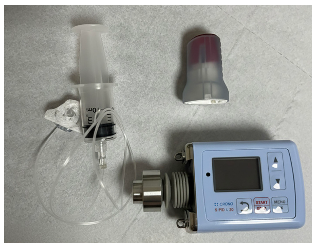
Fig. 1. Photography of the syringe pump, detailing the subcutaneous injection site and the electronic unit.
