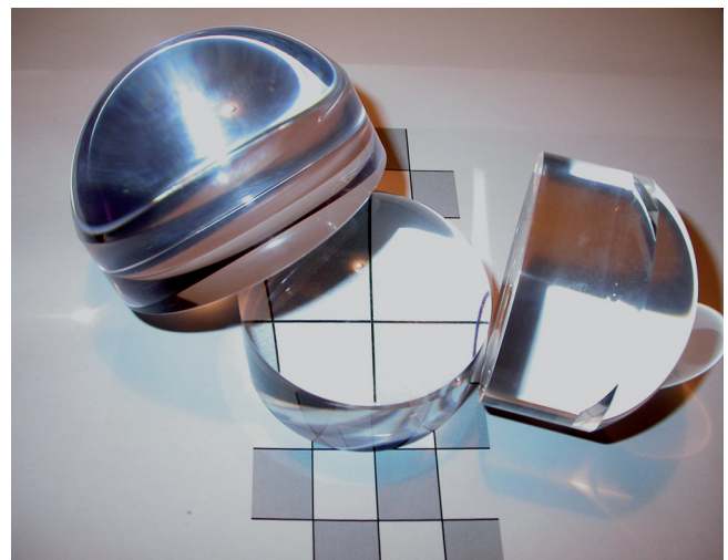
Fig. 1. Globe magnifiers. The globe in the centre is made of acrylic. The magnifying power is easily seen. The globe on left is made of glass, which gives a yellow hue to pictures. The globes consist of a curved surface, which is a converging lens and a cylindrical basis, the height of which equals the focal length of the lens.
