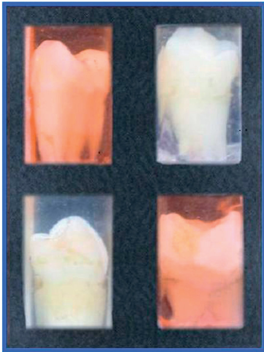
Figure 2. Samples of the teeth embedded in two colours of translucent orthodontic acrylic resin.
