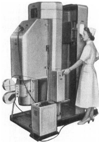
Fig. 4 (a). Photo-fluorographic unit FFS-4 by Schönander.
