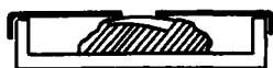
Fig. 1. Cross section of enamel fragment fixed with wax in brass funnel, the exposed area coinciding with lid opening.
