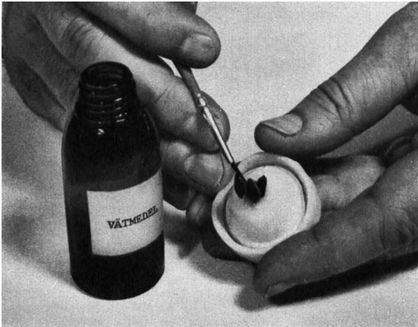
Fig. 6. The wetting agent is brushed over the surface of the pattern.
