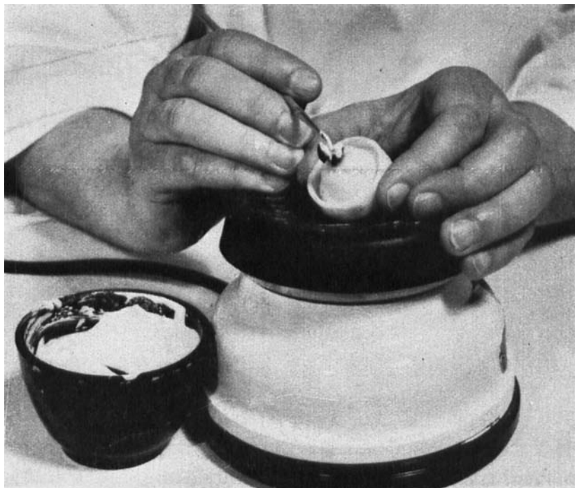
Fig. 7. During vibration the investment is brushed over the pattern.
