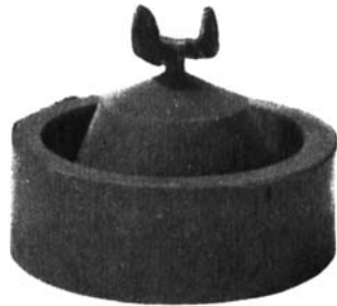
Fig. 5. Rubber cone with finished wax pattern.
