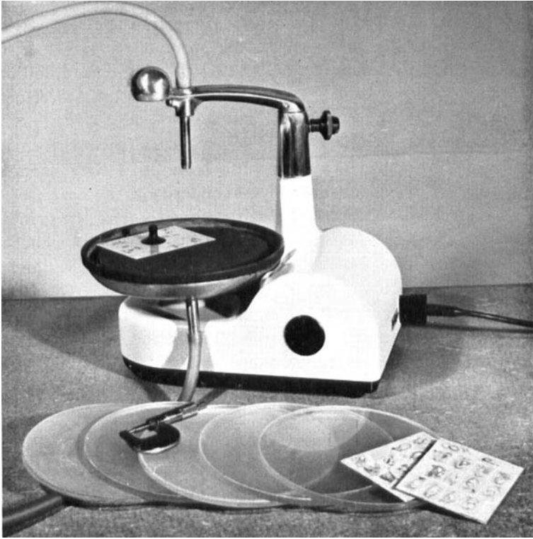
Fig. 1. The grinding apparatus and accessories. On the turntable is the glass plate carrying the abrasive paper. In the foreground are the grinding discs, micrometer gauge and two specimen carriers with sections of jaws of dogs.
