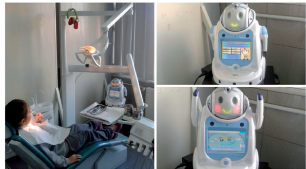
Figure 3. iRobiQ performs some body movements with facial expressions during a child's dental treatment.
