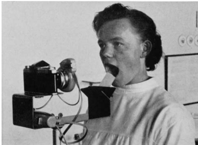
Fig. 1. Photopalatographic apparatus in situ .
