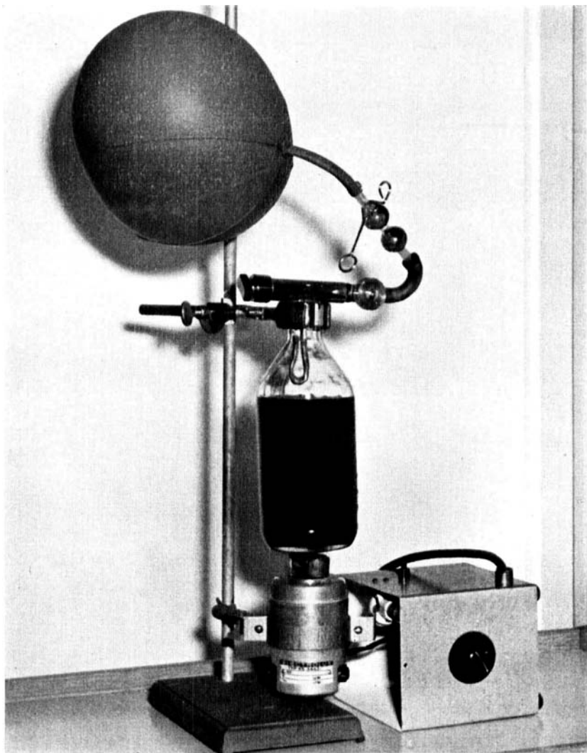
Fig. 1. Arrangement for anaerobic culture in liquid media.
