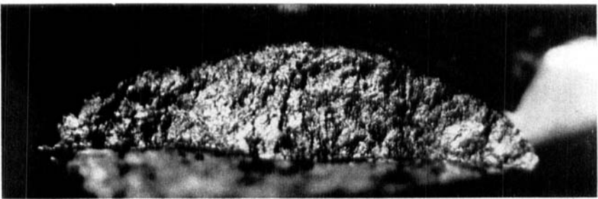
Fig. 7a. Photomicrograph of fracture surface, corresponding to site A in Fig. 1. Magnification x 30. The smooth crystal structure appearing on the surface is due, according to experts, to the effect of hydrogen.
