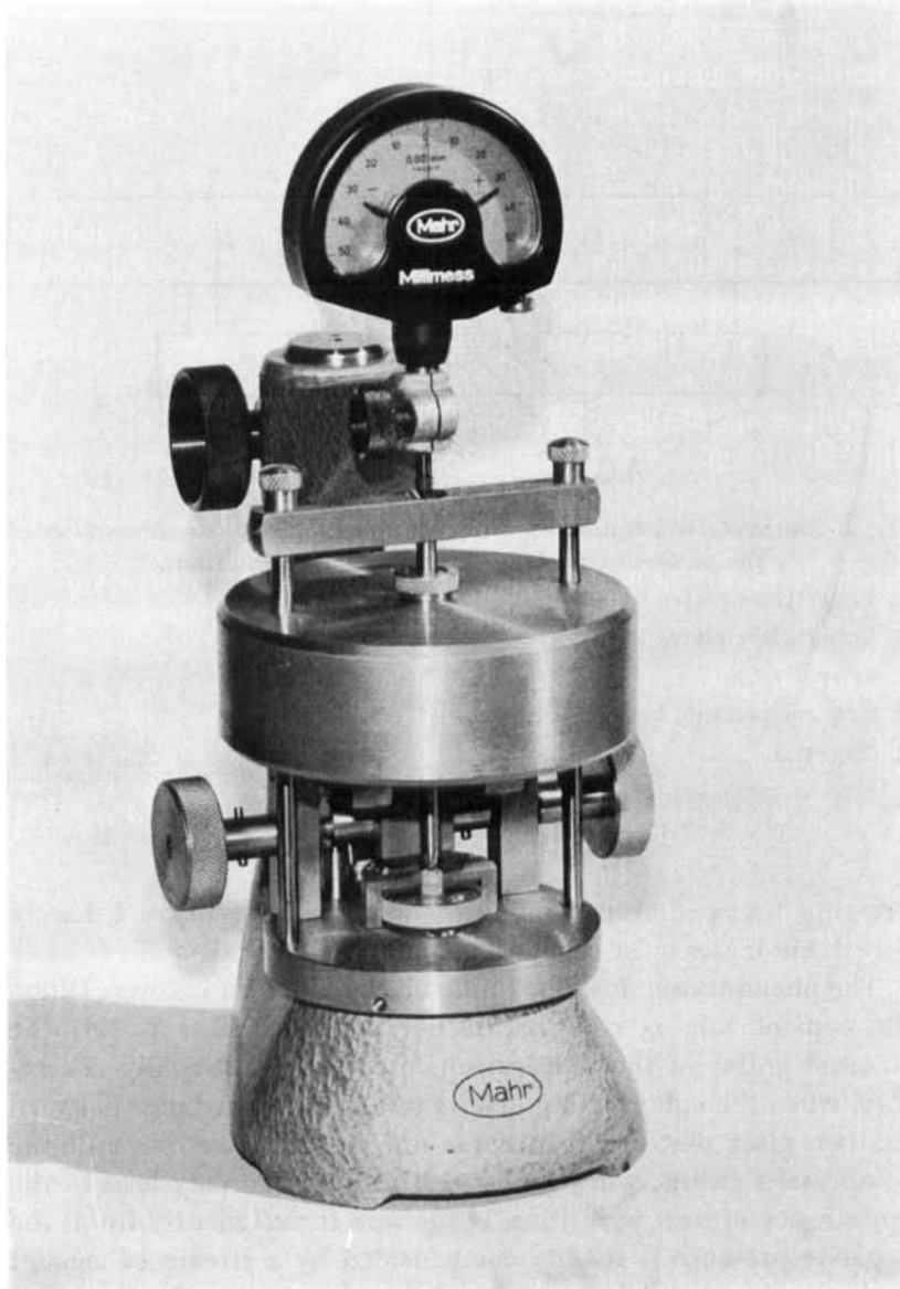
Fig. 1. Equipment for producing thin cement films and for measuring the film thickness.
