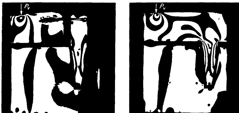
Fig. 15. Stress pattern of a movable saddle (left) and a rigid saddle (right) when a heavy vertical load is applied on the outer end of the saddle resulting in extensive movements. In such cases the movements of the root often cannot be kept within physiologic limits. The rigid anchorage causes greater stress and movements. However, such large movements are not found in superplants (Fig. 12 and 13).
