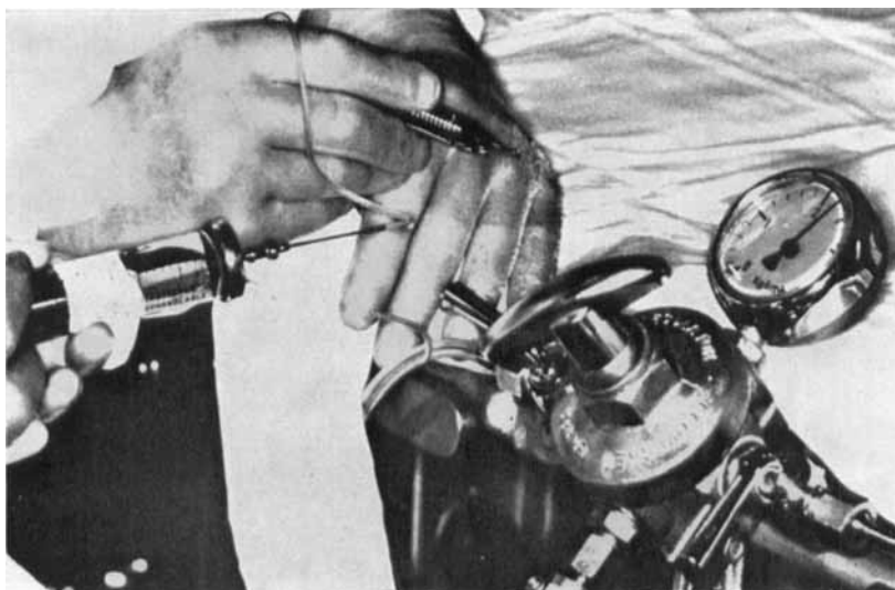
Fig. 7 a. Atlas Copco turbine-powered handpiece connected by a plastic hose to a 20 ml Record syringe, which provides a jet of saline at room temperature on the bur head.
