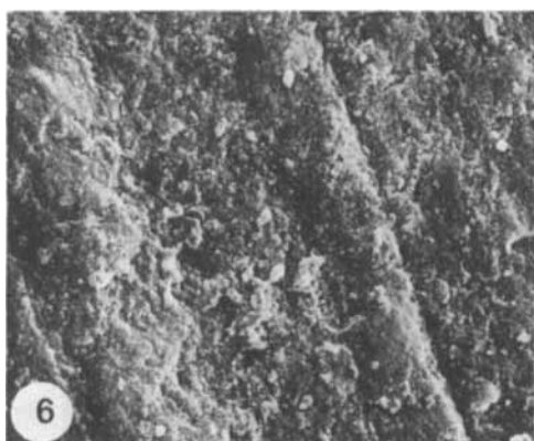
Fig. 6. Dentin polished on paper 800 and rinsed with water. x 3000.
