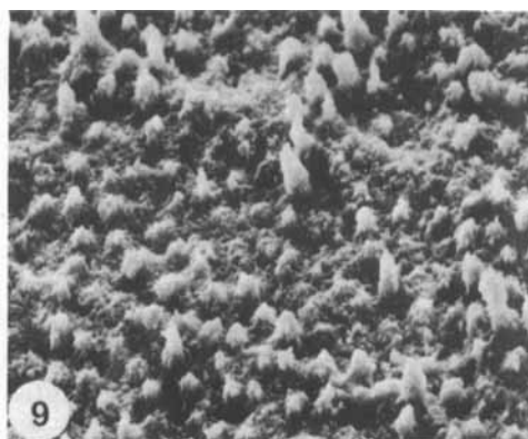
Fig. 9. Composite resin cement after removal from etched dentin. x 1000.
