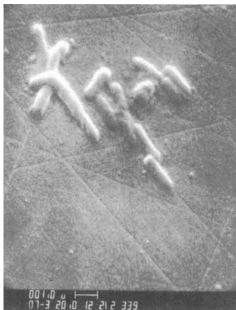
Fig. 10. SEM-picture (x 7000) showing adhering, mostly rod-shaped micro-organisms after two hour intraoral exposure of detergent washed Ge-prism.
