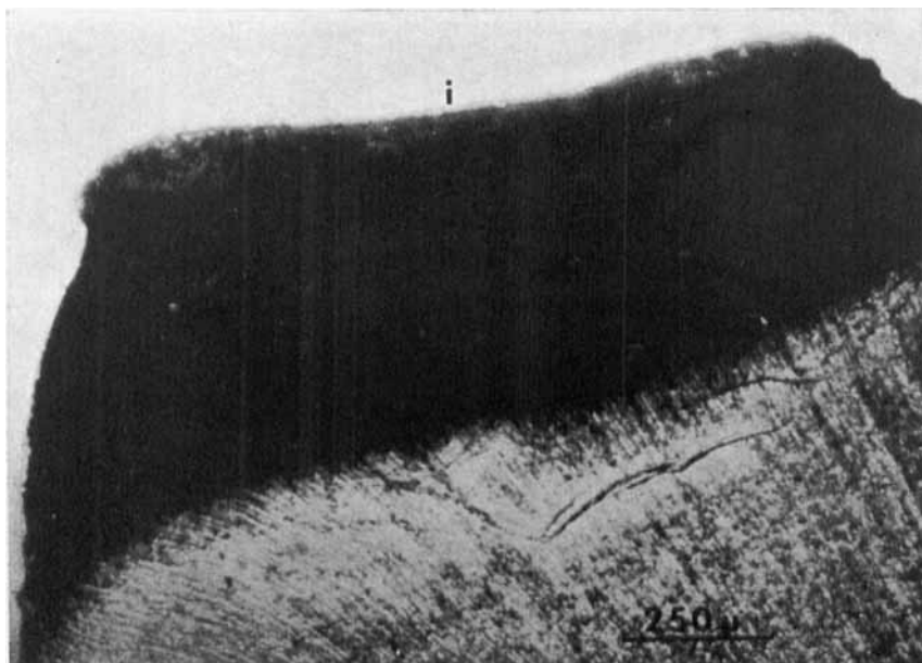
D. Microphotograph in polarized light. Note the negative birefringence (i) and the homogeneous structure in the vicinity of the crater surface.
