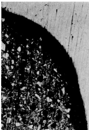
Fig. 2. Marginal fracture in a silicate cement filling. The gap occurring between the filling and the cavity wall due to contraction during setting is clearly visible in the lower right of the marginal area. \times 65 .
