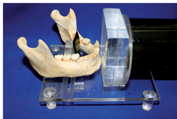
Figure 2. Apparatus used to standardize exposure geometry according to the paralleling technique with an acrylic plate (2.5 cm thick) placed between the X-ray tube and the mandible to simulate soft tissue scatter.
