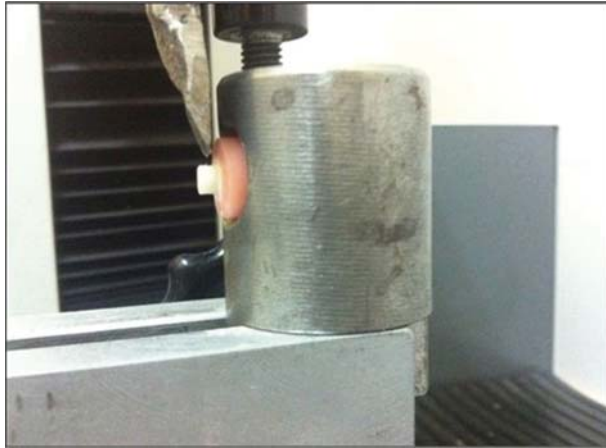
Figure 1. Specimen placed in universal testing machine for shear bond strength test.
