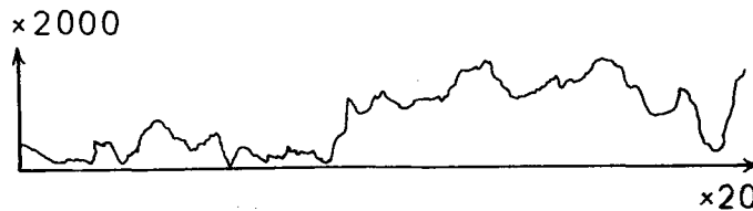
Fig. 4. Graphic profile of a specimen brushed with a dentifrice of medium abrasive effect, no. 6.
