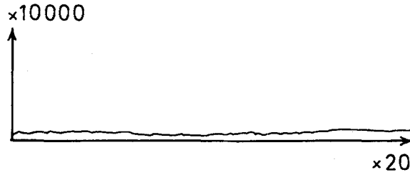
Fig. 3. Graphic profile of a specimen brushed with a dentifrice of low abrasive effect, no. 1.
