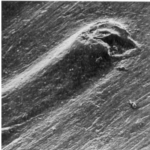
Fig. 9. An irregularity of the polymerized acrylic surface can be developed to a pit with a ridge. (dentifrice no. 2, \times 500 ).
