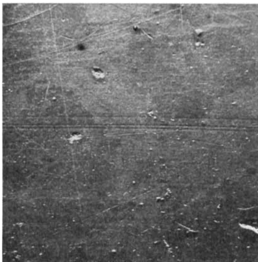
Fig. 6. Acrylic surface brushed with dentifrice no 1. No scratch marks noticed (SEM-photogram \times 500 ).
