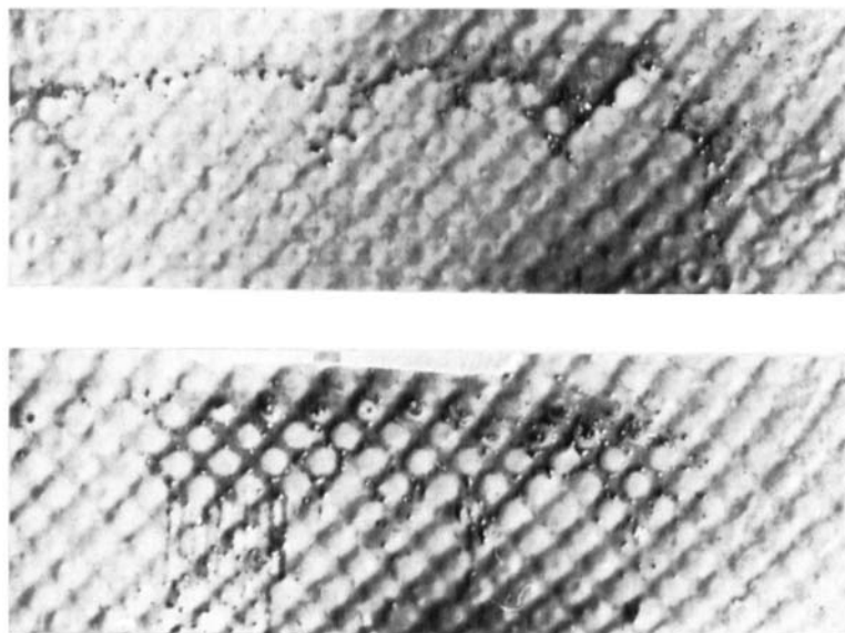
Fig. 3. Droplets of mercury on adhesive plaster which was wound around leaking capsules during mechanical trituration. The top plaster represents a mercury loss of 9 mg, the lower plaster a loss of 20 mg. Approx. twice actual size.
