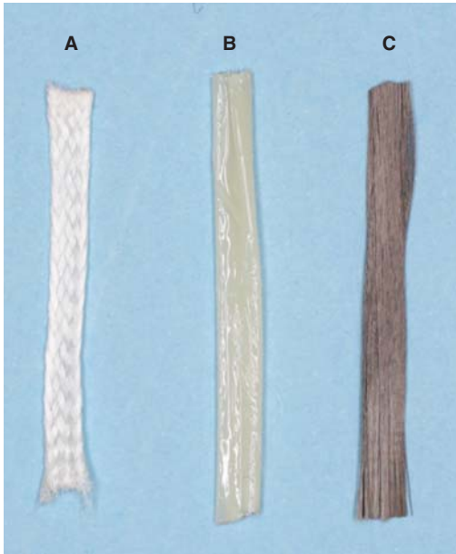
Figure 1. Types of fibers used to reinforce resin composites in this study: (A) Polyethylene fiber; (B) Glass fiber; and (C) Carbon fiber.
