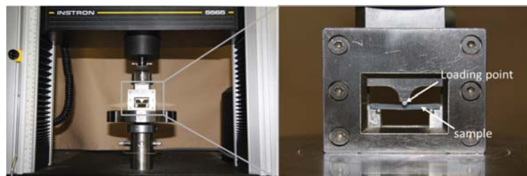
Figure 2. Static three-point flexural test set-up. Resin composite specimen was mounted on test jig.
