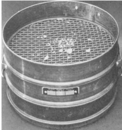
Fig. 1. Sieve-system, consisting of 3 sieves with meshes of 5.6, 4.0 and 2.0 mm
