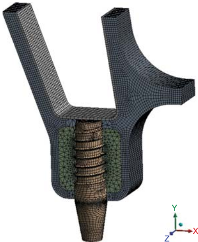
Figure 1. Finite element model of sinus area bi-cortical dental implantation with bone containing nodes and elements. Sample Model 1–2 with 1 mm thickness crestal cortical bone and 1 mm sinus floor cortical bone and standard implant bi-cortical implantation in the sinus area.
