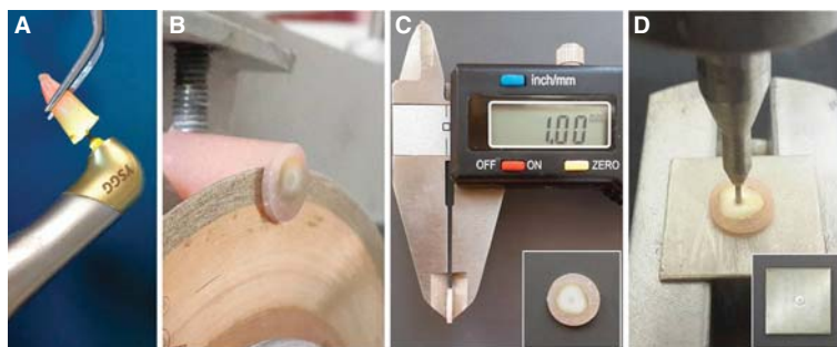
Figure 1. Experimental set-ups images. (A) laser application, (B) a post/dentin slice section process, (C) actual length measurement, (D) compressive load application.
