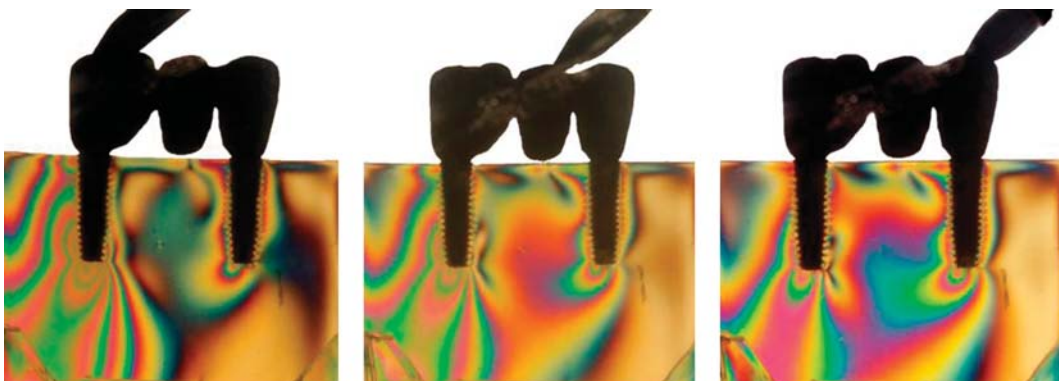
Figure 8. Oblique load for Group II, applied in three different points.
