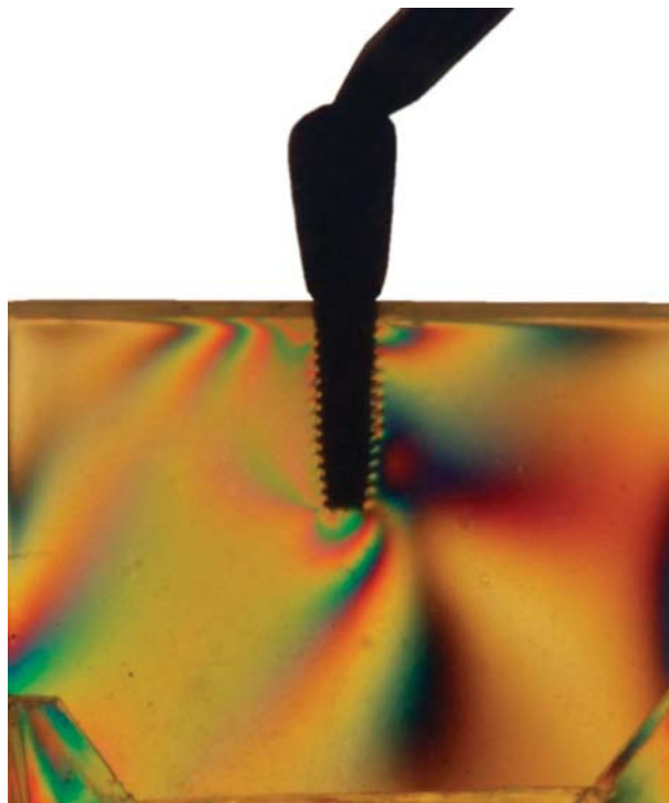
Figure 7. Axial load for Group II, applied in three different points.
