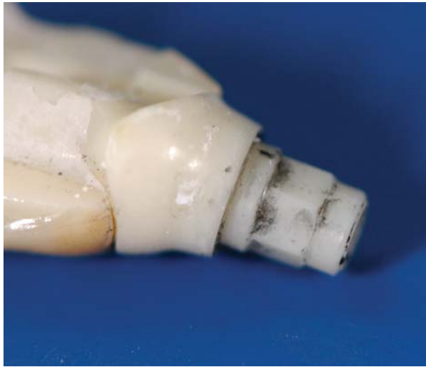
Figure 1. Image of a removed abutment after 2 years in function, which showed a screw loosening and rotational misfit. Residual titanium debris is visible in the area of the internal hexagonal connection geometry.
