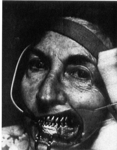
Fig. 8. Test person prepared for holography. The region to be exposed is covered as described separately with special paint for total reflexion of the laser light. The subminiature force sensor is positioned between 24 and its opposing teeth. During the registration of the hologram the eyes of the patient are protected by means of black glasses.
