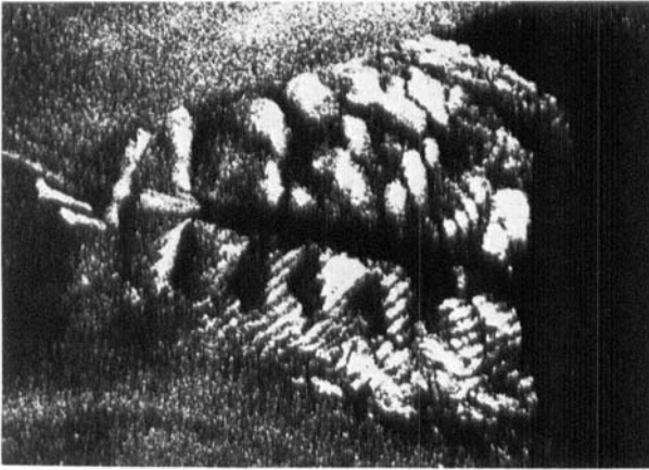
Fig. 11. Photographed holographic reconstruction of the exposed jaw section. The interference fringes indicate the mobility and deformation caused by the force increase between the laser pulses.
