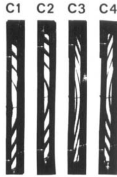
Fig. 10. Photographed reconstructions of holograms. Test bars C 1—C 4 are on a two-edge support. The between-exposure force application is 1.5 N. The basic force level is 3.0 N. The interference fringe pattern reveals the deflection as well as a slight torsion within the bars during the experiment. White arrows indicate the positions of edge support.
