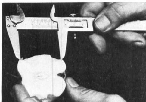
Fig. 2. Measuring of the distance between the impressions in the apple of the upper and lower teeth using a sliding caliper.
