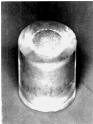
Fig. 26. Corrosion due to the presence of a concentration cell element between the free surface of amalgam and the surface against a glass tube. 3 \times .
