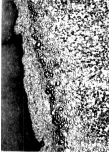
Fig. 30. Drops of free mercury along the margin of a section through a corroded amalgam filling. 90 \times .
