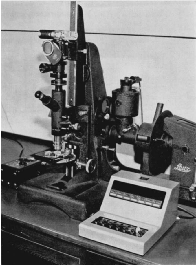
Fig. 3. Point counter mounted on the Panphot microscope together with Ultropak objective.
