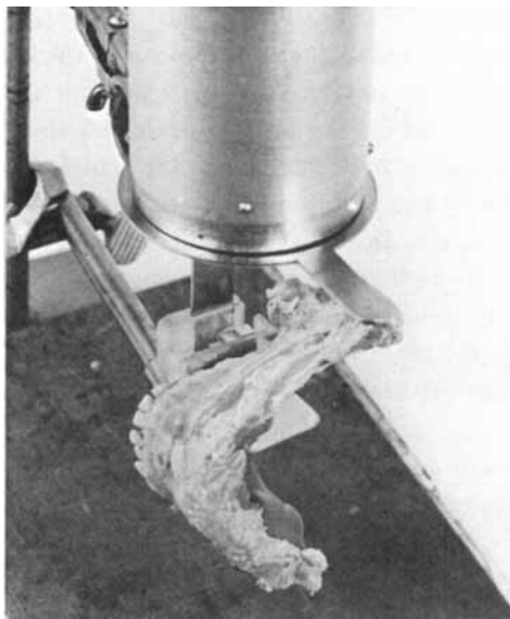
Fig. 6. Roentgen tube, film holder and jaw mounted in a rigid system. The film can be changed without disturbing these relationships.
