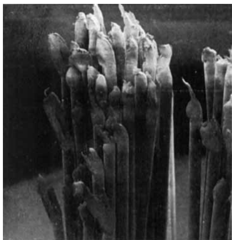
Fig. 1. Bristles from a new nylon toothbrush. There are 50 bristles in each tuft. The length of the bristles varies between 9 and 13 mm. The diameter of each bristle is approximately 0.25 mm. Scanning EM. \times 22 .
