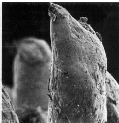
Fig. 2. The ends of the bristles of a new nylon toothbrush. The bristles are sharp due to the oblique cutting. The bristles have an even thickness and a cross-section in the form of a circle. Scanning EM. \times 220 .
