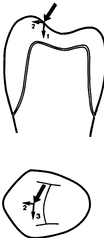
Fig. 2. The load on an artificial crown divided in three force components:
