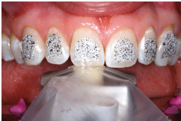
Figure 1. Extraoral anterior view of the experimental set-up of vertical load application. The magnet retained loading device maintained in position by a metal plate that is attached to the mandibular teeth by silicone material. For hygiene reasons the load device is covered with a single-use plastic cover. Adhesive tape with a stochastic surface pattern is fixed on all six anterior teeth. Surface pattern is tracked by digital image correlation system over all load stages.
