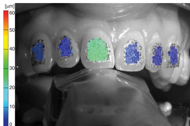
Figure 3. Anterior screen image of surfaces as calculated by the measurement system during load application. Tooth displacement was measured against reference areas on adjacent unloaded teeth (blue areas). Tooth displacement at 9 N is shown as an example (see color scale).
