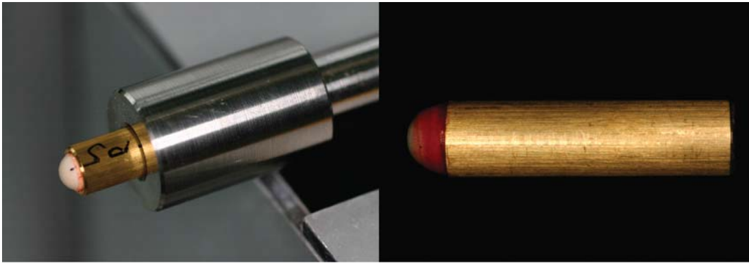
Figure 2. Left: Steatite ball in the messing sleeve; Right: Holder of the sleeve with integrated steatite ball, which represents the antagonist.
