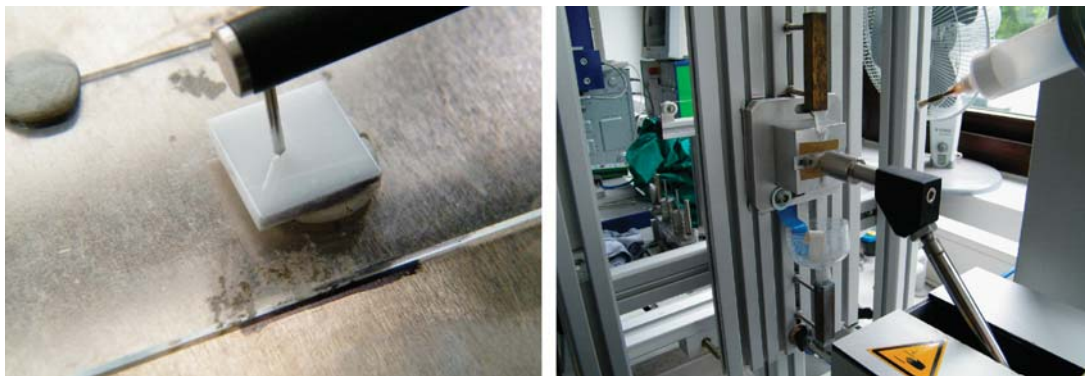
Figure 1. Left: the Perthometer S6P. All specimens were topographically recorded over a surface area of 3 × 3 mm with 121 profiles; right: the Abrex-Apparature.
