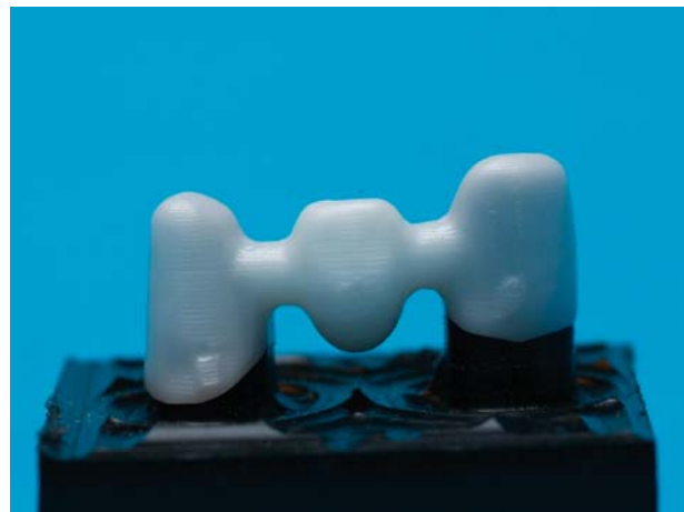
Figure 4. Y-TZP FDP cemented on acrylic tooth-supporting analogue.
