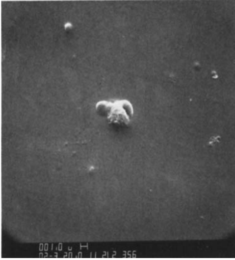
Fig. 9. SEM-photograph (original magnification 200 X) showing particle adhering to film covered Ge prism at the end of a 2 hr unprovoked intraoral exposure. Simultaneously performed dispersive x-ray analysis gave the following most prominent absorption bands: 1.186 keV (Ge L\alpha -band); 2.308 keV (S K\alpha -band); 2.838 keV (Pd L\alpha -band); 3.690 keV (Ca K\alpha -band); 4.012 keV (Ca K\beta -band); 9.885 keV (Ge K\alpha -band); 11.100 (Ge K\beta -band).
