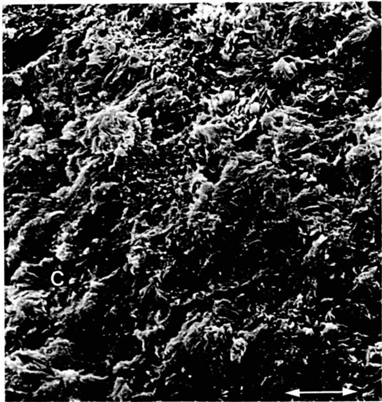
Fig. 8. In the nucleus the fracture surface had a fine granulated mineralized structure with crystallization centers with crystals radiating from a core (C). Arrows equal 5 \mu m.
